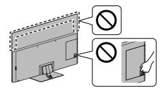
Transport only in upright position. Transporting the TV with its display panel facing upwards or downwards may cause damage to the internal circuitry.
